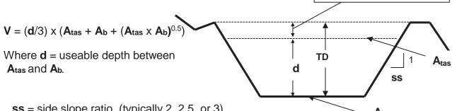
ss = side slope ratio. (typically 2, 2.5, or 3)
