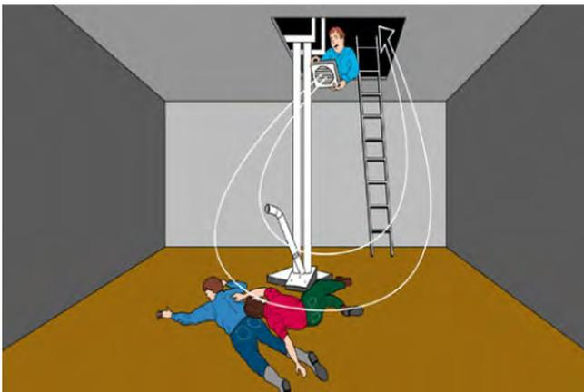
Keeping the fan outside the space reduces this risk. Also be alert that gas that is being blown out of the space does not blow directly back toward you. If the confined space is a relatively small enclosed tank, the gas might be coming back out the opening where you are holding the fan. Make sure you are not exposing yourself to this potentially toxic air.
