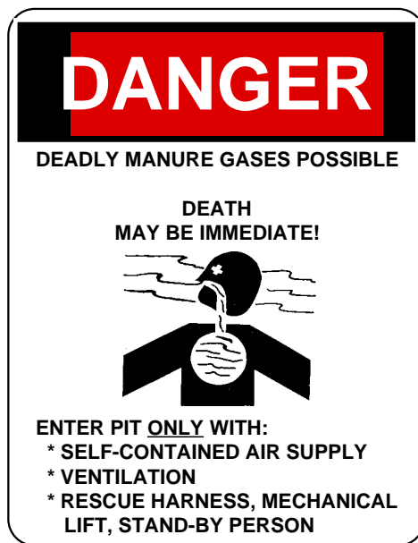
Figure 1. Warning signs such as this example should be placed at all entrances to manure storage pits.
